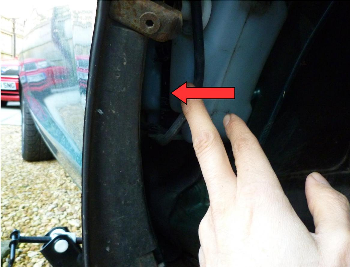
Now the pump and filter have to be removed from the bottle – this is the tricky part of the job and requires patience and a bit of dexterity. If you are carrying out this job in order to replace the pump, then remove the electrical connector at the top of the pump and the hose connection at the bottom. If you are carrying out the job in order to clean a suspected blocked filter then leave these items in place.
